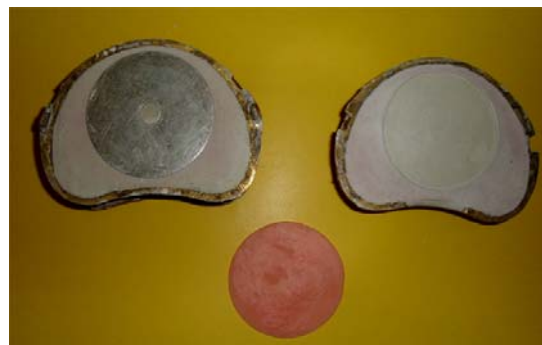
Figure (1) : Acrylic resin disk for water sorption and solubility test.
