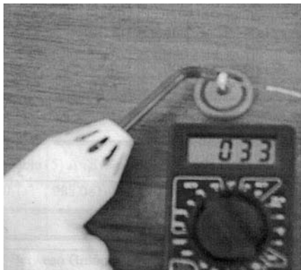
Figure (1): Quartz tungsten halogen curing unit "Astralis", tooth sample and the Digital Multimeter
